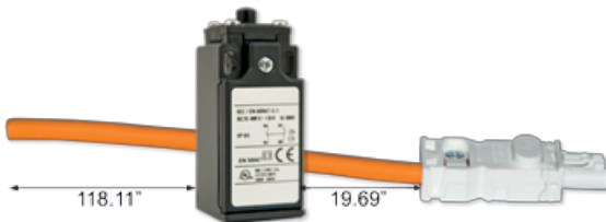
Connection cable 2 x AWG 18, halogen free with door switch and Wieland female connector. NC wired, strain release, mounting plate for door switch
